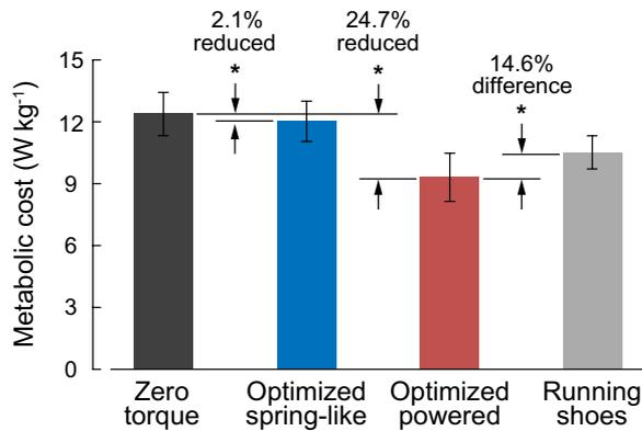
**Fig. 2. Metabolic results.** Optimized spring-like and Optimized powered assistance resulted in metabolic reductions of 2.2 and 24.7%, respectively, compared with zero-torque mode, while running at  $2.7 \text{ m s}^{-1}$ . Optimized powered assistance resulted in an improvement in running economy of 14.6% compared with running in normal shoes, whereas Optimized spring-like assistance resulted in an 11.1% increase in the energy cost of running. Error bars indicate SD. \* $P < 0.05$ .
