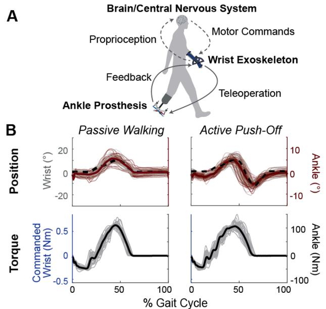
**Figure 1: A.** We use a wrist exoskeleton to both control and receive haptic feedback from an ankle-foot prosthesis to restore the motor control loop. **B.** The two desired trajectories with haptic feedback are shown, in addition to how well the wrist and ankle matched these trajectories and the resulting torque profiles. The dashed line indicates the desired trajectory, and bold lines indicate averages.
