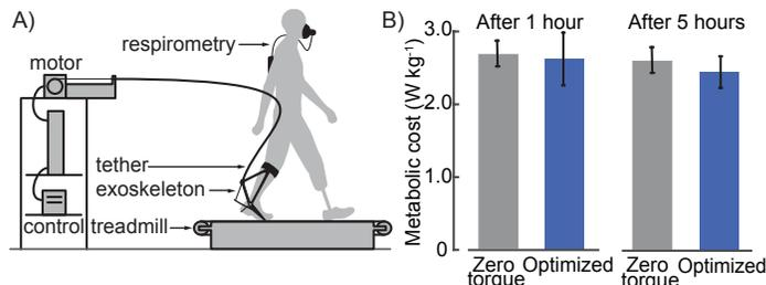
**Figure 1:** A) Exoskeleton emulator system, with the device worn on the sound limb of people with unilateral amputation. B) Average metabolic cost of users after approximately 1 and 5 hours of optimization, during the zero torque and optimized assistance conditions.
