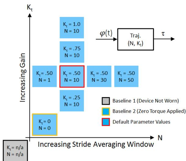
**Figure 3.** Experimental protocol of parameter sweep. Gain ( $K_t$ ) and stride averaging window  $N$  will be independently varied from default values (outlined in red) in a randomized series of trials to determine the effects of these parameters on the controller’s dynamic calculation of torque.
