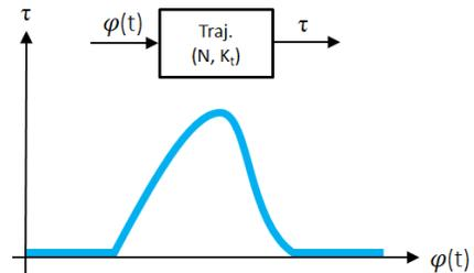
**Figure 2.** Control architecture of joint torque trajectory control. The torque generated is a scaled ( $K_t$ ) function of current stride phase  $\varphi(t)$  normalized via a filtered average over the last  $N$  stride periods.
