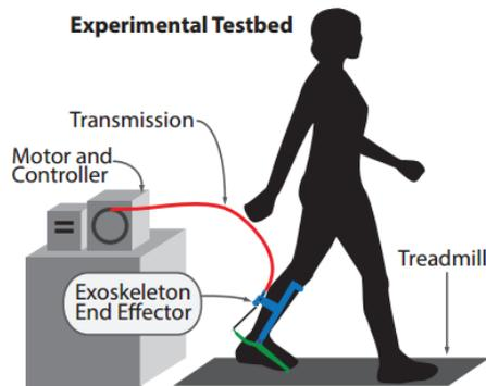
**Figure 1.** Depiction of experimental testbed during unilateral AFO testing. An off-board motor and controller control the exoskeleton end effector via a Bowden cable transmission. Tests are conducted with able-bodied subjects on a split-belt force-sensitive treadmill.
