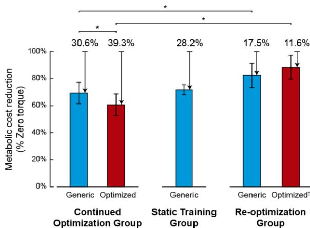
**Figure 1:** Metabolic costs of exoskeleton walking under different types of training, with respect to a zero torque condition. The optimized assistance for individuals in the continued optimization group resulted in the largest reduction in metabolic cost by any exoskeleton to date. The response to the generic condition was significantly worse for the re-optimization group compared to the continued optimization group, suggesting that too much variation can interfere with training.
