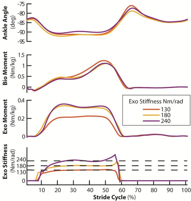
**Figure 1:** Gait dynamics and ankle exoskeleton emulator (Exo) performance across three stiffness conditions during walking at 1.25 m/s. Dashed lines indicate the desired exoskeleton rotational stiffness.
