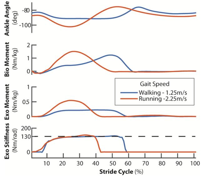
**Figure 2:** Gait dynamics and ankle exoskeleton emulator (Exo) performance for walking (1.25m/s) and running (2.25 m/s) at a desired exoskeleton rotational stiffness of 130 Nm/rad. Dashed lines indicate the desired rotational stiffness.
