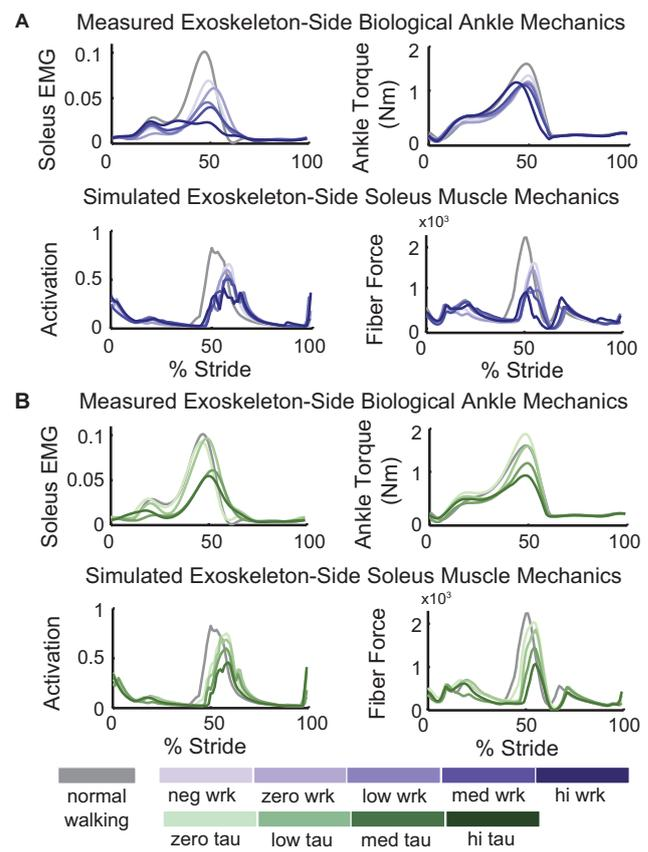
**Figure 1:** Preliminary results for one subject across A) work conditions and B) torque conditions. Top row of A) and B), from left to right, shows experimentally-measured exoskeleton-side soleus electromyography and biological ankle torque. Bottom row, from left to right, shows simulated exoskeleton-side soleus activation and fiber force. Normal walking is in grey. Work conditions are in purple, torque conditions are in green, and darker colors indicate higher values.
