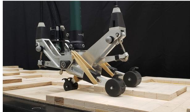
Fig. 1. The prosthesis emulator adapting to an uneven surface.
