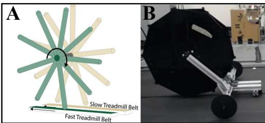
**Figure 1:** Split-Belt Rimless Wheel Model. A: Simulation Model B. Physical Prototype
