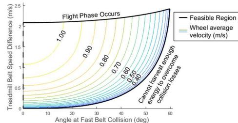
**Figure 2.** With an infinitesimally small angular offset between the plates such that collision onto the slow belt occurs at nearly vertical, the model can walk steadily with a large range of inter-leg angles and treadmill speed differences. Results look similar as the offset increases as long as the fast collision angle remains significantly wider.
