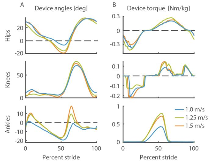
**Figure 2:** Average exoskeleton joint angles and optimized, exoskeleton torques. (A) Average hip, knee and ankle device angles during optimized torque application. (B) Average applied hip, knee and ankle torque. The applied torques at the hip and ankle are torque-time profiles, and the applied torque at the knee is defined by a virtual spring during stance, time based flexion near toe off a virtual damper during late swing.
