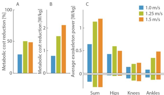
**Figure 1:** Metabolic reduction and exoskeleton power after optimization at all three speeds. (A) Metabolic reduction normalized to metabolic cost of walking with the device turned off. (B) Absolute metabolic reduction relative to walking with the device turned off. (C) Average positive and negative joint power at the hips, knees, ankles, and sum of all three. The y-axis scale for C is half the scale of B.
