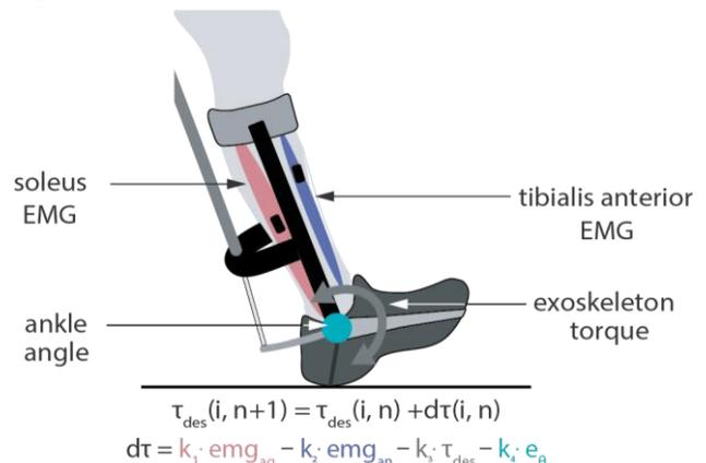
Figure 2. Overview of the heuristic based controller [3].
