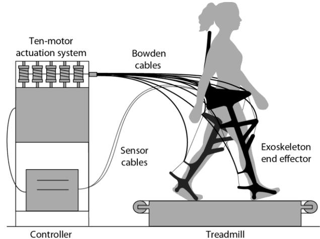
Figure 1. Schematic of the exoskeleton emulator system.
