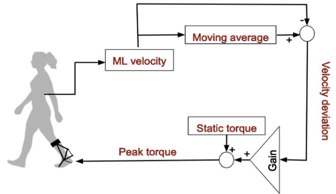
Figure 1: High-level controller used to modulate ankle push-off torque.
